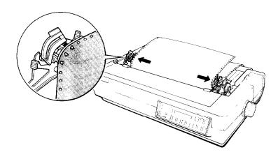
7. If the paper does not fit exactly onto the tractor pins, press in on the pull tractor feed knob and turn it in the desired direction.
